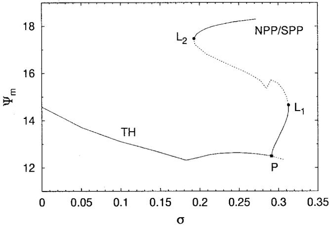
Figure 9. Bifurcation diagram for the rotational case with full wind stress. Note the shift of the pitchfork bifurcation  $P$  to larger values of  $\sigma$ , opening a large window where multiple equilibria exist.
