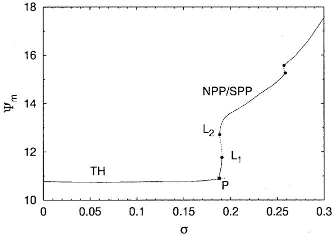
Figure 6. Bifurcation diagram in the control parameter  $\sigma$  for the case of full rotation ( $\eta_f = 1$ ) and parameters similar to those of Figure 2. The PP branches lose their stability at the limit point  $L_1$ , but regain stability at  $L_2$ . The limit points close to  $\sigma = 0.25$  reflect minor rearrangements of the steady state patterns.
