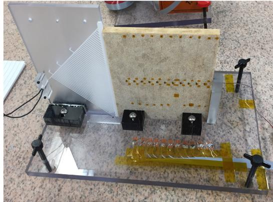
Fig. 1: Shot 8-1940 assembly. Detonation in the slab was initiated by a Teledyne-Risi RP-2 detonator and a line-wave generator. Ionization wires are visible along the centerline of slab and a font curvature window is at the center of the breakout surface.
