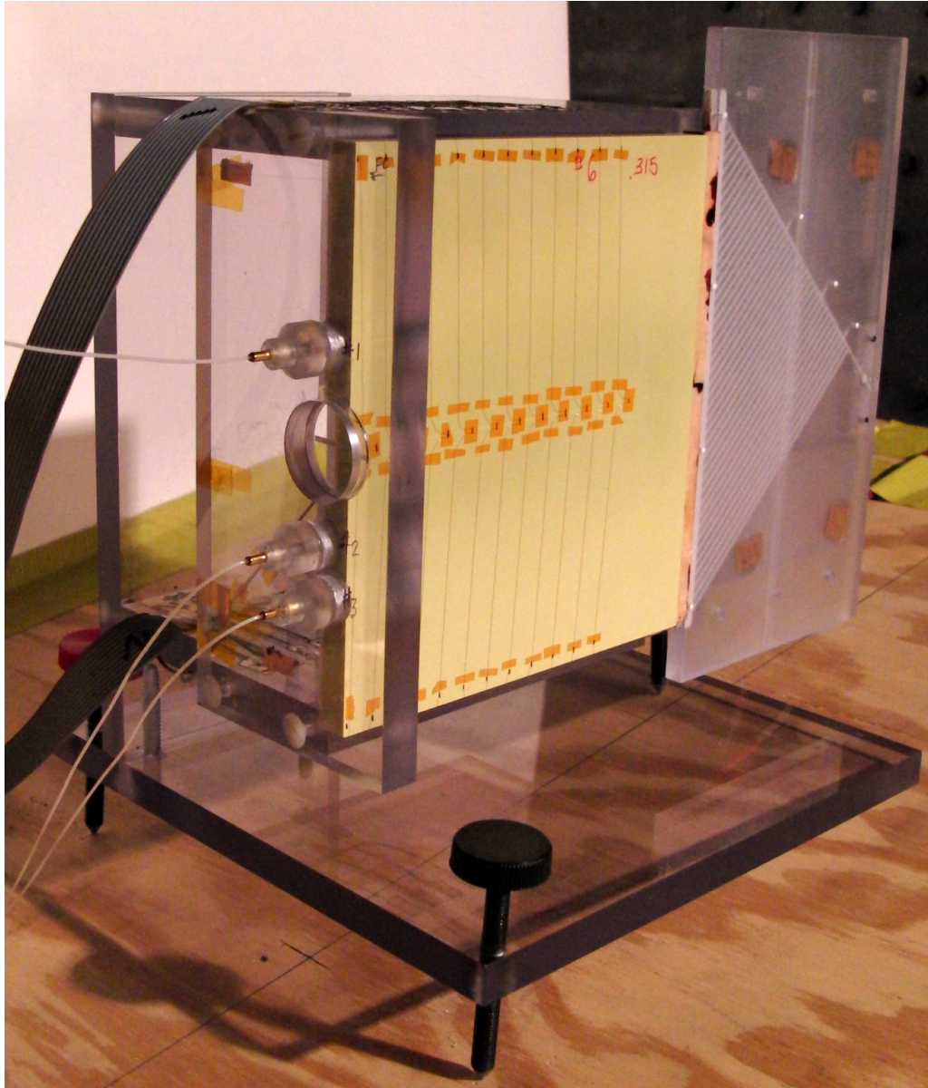
Figure 4: Perspective view showing the PBX 9502 side of explosive assembly.
