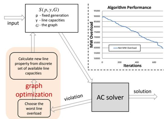
Figure 4: The Abstract Network Design Optimization Algorithm and sample algorithm output.
