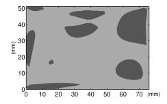
Fig. 8 – Diagram of points were the physical experiment met (light gray) and did not meet (dark gray) the acceptance criteria of the mean residual stress falling within the bound of the measured stress  $\pm$  total uncertainty (68% confidence interval); 72% of points meet the acceptance criterion
