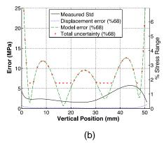
Fig. 7 – Line plots of the measured standard deviation, displacement error, model error, and total uncertainty in the (a) horizontal direction at the mid-thickness (y = 25.4 mm) and (b) vertical direction at the mid-width (x = 38.1 mm)
