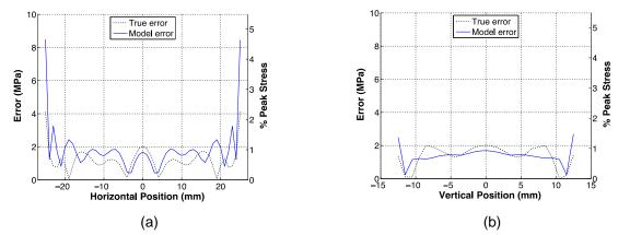
Fig. 4 – Line plots of the model error and true error in the (a) horizontal direction at the midthickness (y = 0) and (b) vertical direction at the mid-width (x = 0)
