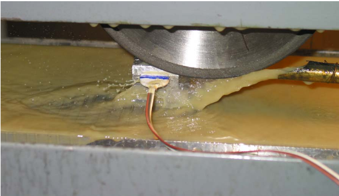
Figure 3. The test specimen during the slitting process.
