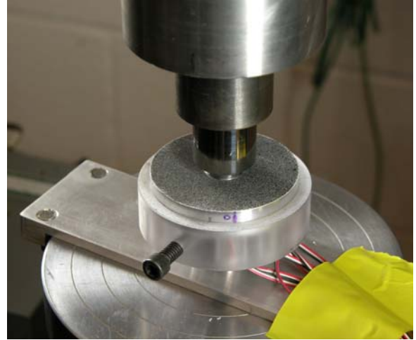
Figure 7 The disk specimen shown during the indentation test. The DIC speckle pattern is visible on the top face of the disk.
