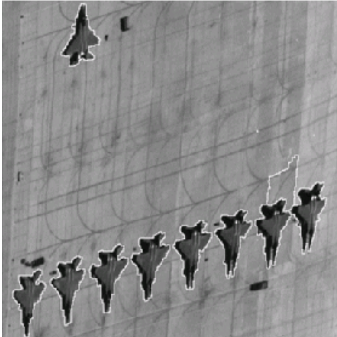
Fig. 5. Watershed Algorithm. A watershed algorithm produced a comparable segmentation of the original image, although a spurious feature on the tarmac was also extracted.
