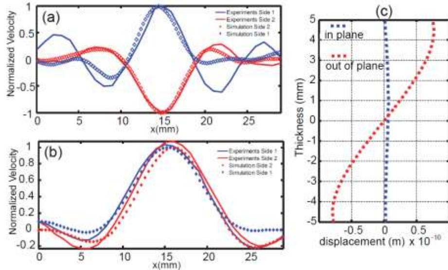
Fig.2. Comparison experiment/numerical at Z1. (a) Symmetric and (b) antisymmetric mode focusing. (c) Numerical wave structure (displacements) over the thickness of the plate for the symmetric mode.
