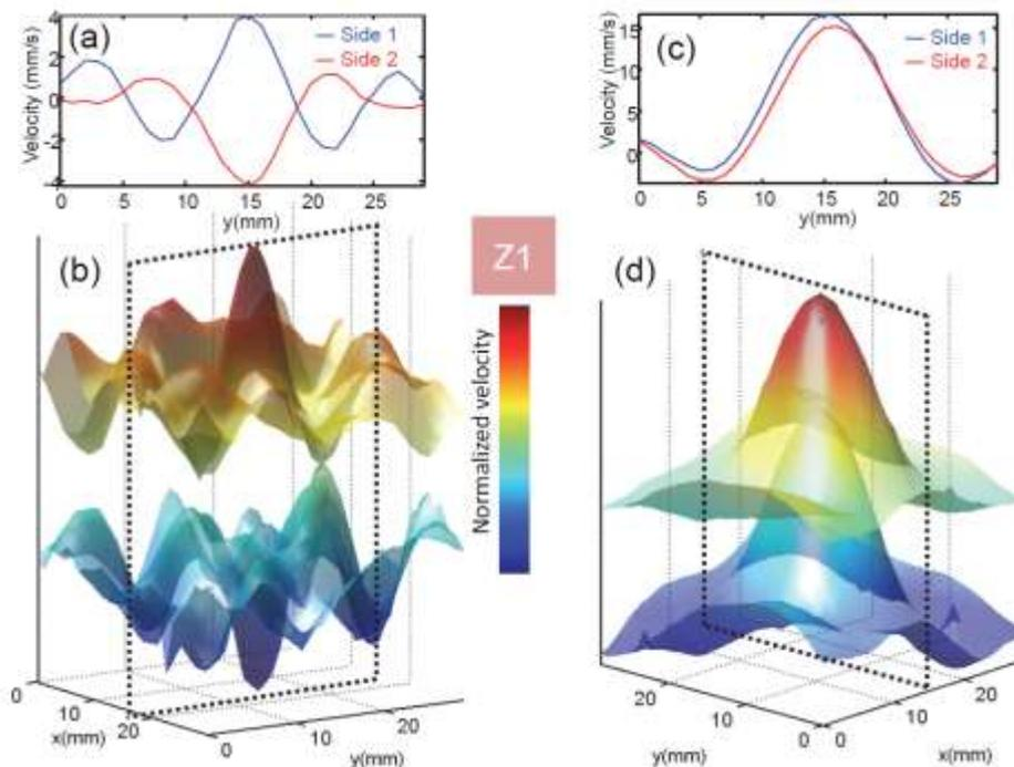
Fig. 3. Experimental focusing in Z1 zone. Left panel: Symmetric mode focusing, with the particle velocity map on the bottom and a slice on the top. Right panel: Antisymmetric mode focusing, with the particle velocity map on the bottom and a slice on the top.
