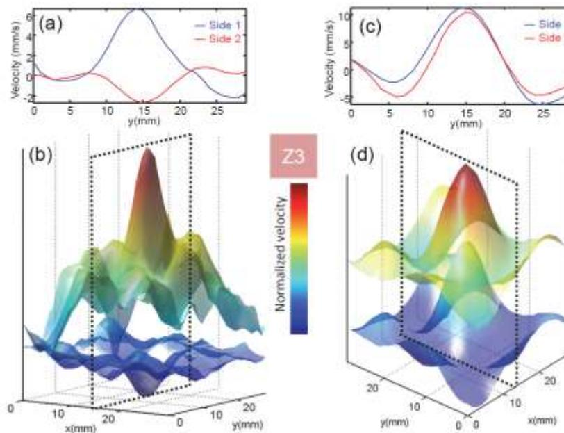
Fig. 5. Experimental focusing in Z3 zone. Left panel: Symmetric mode focusing, with the particle velocity map on the bottom and a slice on the top. Right panel: Antisymmetric mode focusing, with the particle velocity map on the bottom and a slice on the top.
