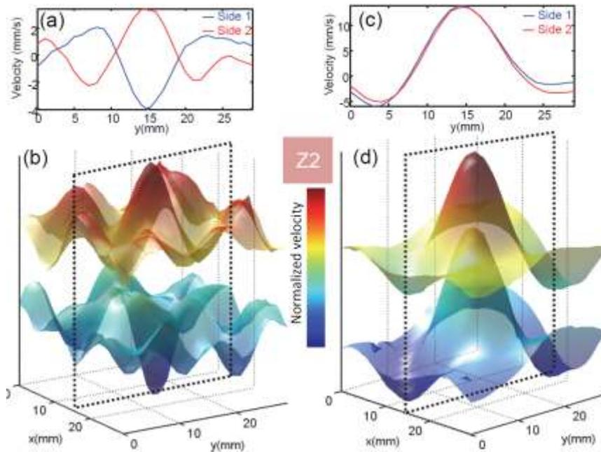
Fig. 4. Experimental focusing in Z2 zone. Left panel: Symmetric mode focusing, with the particle velocity map on the bottom and a slice on the top. Right panel: Antisymmetric mode focusing, with the particle velocity map on the bottom and a slice on the top.
