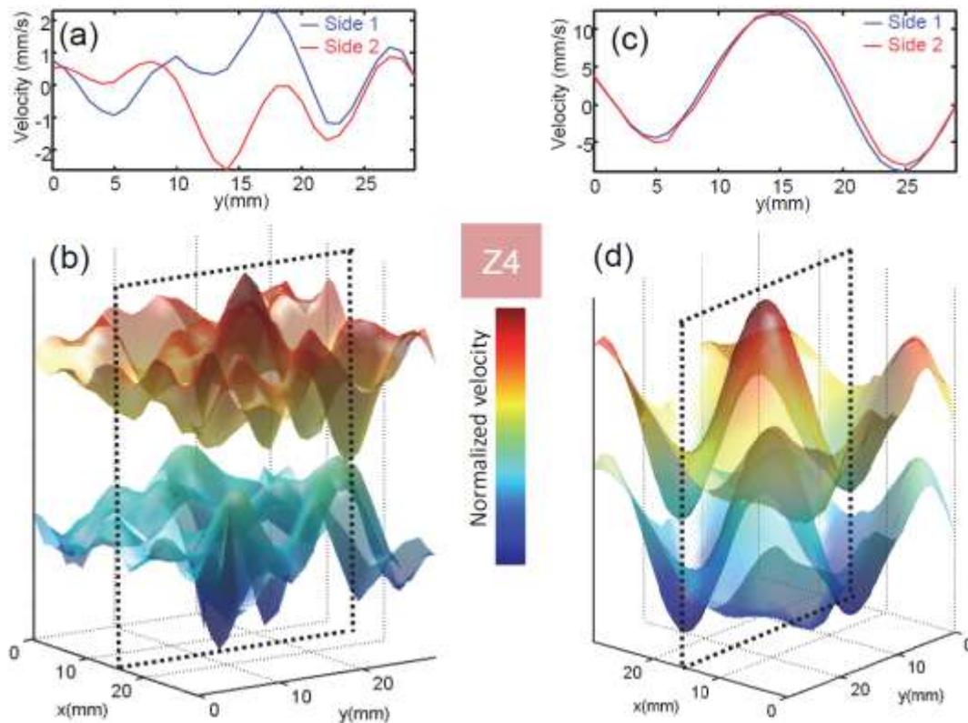
Fig. 6. Experimental focusing in Z4 zone. Left panel: Symmetric mode focusing, with the particle velocity map on the bottom and a slice on the top. Right panel: Antisymmetric mode focusing, with the particle velocity map on the bottom and a slice on the top.
