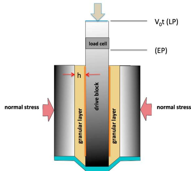
**Figure 1.** Apparatus of the biaxial experiment. The load cell has an effective stiffness  $k$  (see equation (4)); the load point (LP) is displaced at a constant speed  $v$ ; the displacement of the EP is denoted by  $x$  in equation (4). The granular layer is subject to a normal stress  $p$  which is held fixed except when going from one stress step to another.
