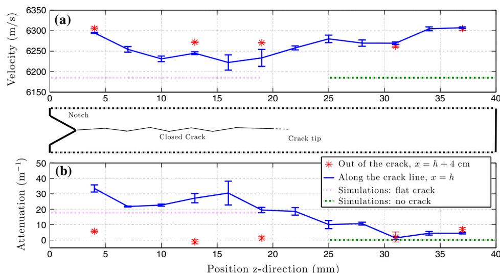
**Fig. 2** Ultrasonic propagation: linear velocity and attenuation measurements. **a** Velocity as a function of the position along the crack ( $x = h$ ). Red stars represent velocities measured far from the crack, along the width corresponding to  $x = h + 4\ \text{cm}$ , for comparison. Simulation results are also presented for comparison (no crack and flat crack cases). **b** Attenuation as a function of the position along the crack. The
