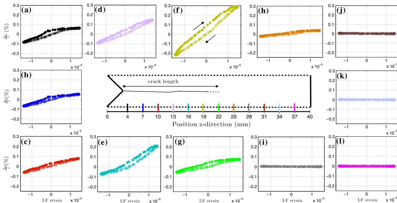
**Fig. 6** DAE results for 12 different positions along the sample width  $L_z$ . Relative velocity change  $\frac{\Delta v}{v}$  is represented as a function of low frequency strain  $\epsilon_x$ . Positive (negative) strain corresponds to tension (com-
