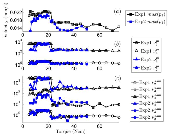
FIG. 4. (Color online) Evolution of foci’s maxima and associated nonlinear parameters vs torque, expressed in N · cm, for two experiments. (a) Maximum of the focus  $p_1$ . (b) Evolution of nonlinear parameters  $\nu_2^{pi}$  and  $\nu_4^{pi}$ . (c) Evolution of nonlinear parameters  $\nu_2^{ssm}$  to  $\nu_4^{ssm}$ .
