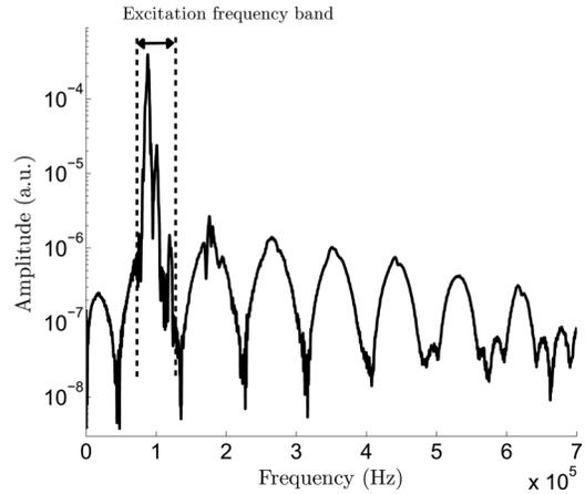
FIG. 6. Spectrum of the focus signal  $p_1$  for a 10 N·cm-torque. We observe the presence of both odd and even harmonics without predominance of odd harmonics. This observation supports primarily a nonlinear “classical” regime that is taken into account for the normalization of  $\kappa$  parameters.
