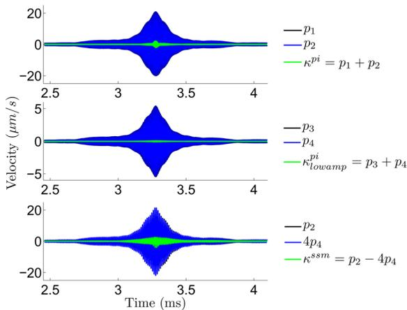
FIG. 2. (Color online) Time foci measured at 10N · cm and nonlinear components extracted from these foci vs time. (a) Recorded signals  $p_1$  and  $p_2$ , as well as the nonlinear component  $\kappa^{pi}$ . (b) Recorded signals  $p_3$  and  $p_4$ , as well as the nonlinear component  $\kappa_{lowamp}^{pi}$ . (c) Recorded signals  $p_2$  and  $p_4$ , the latter being rescaled by a factor 4, and the nonlinear component  $\kappa^{ssm}$ .
