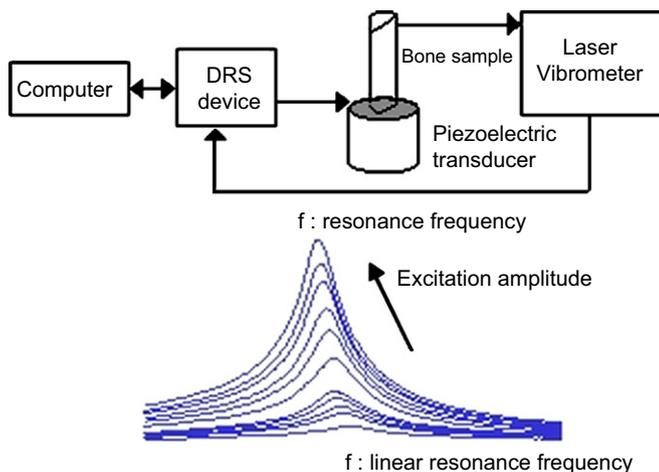
Fig. 1. Top: Nonlinear Resonant Ultrasound Spectroscopy setup. Bottom: frequency response of one sample for increasing excitation amplitudes. The resonance frequency decreases as drive amplitude increases in damaged samples.
