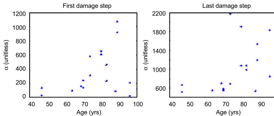
Fig. 3. Evolution of the nonlinear parameter  $\alpha$  as a function age for all the tested samples. An exponential relationship was found between the two parameters. Note that an exponential relationship had also been found in a previous study between age and micro-crack density (Schaffler et al., 1995).
