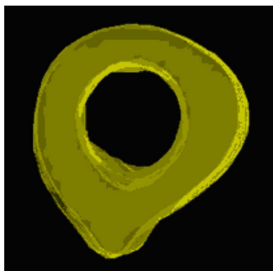
FIG. 1. (Color online) Cross section of the sample, a 6 cm tall (out of the plane of the figure) section of cortical bone taken from a human diaphysis (femur). The average outer diameter of the cross section is approximately 2.5 cm.
