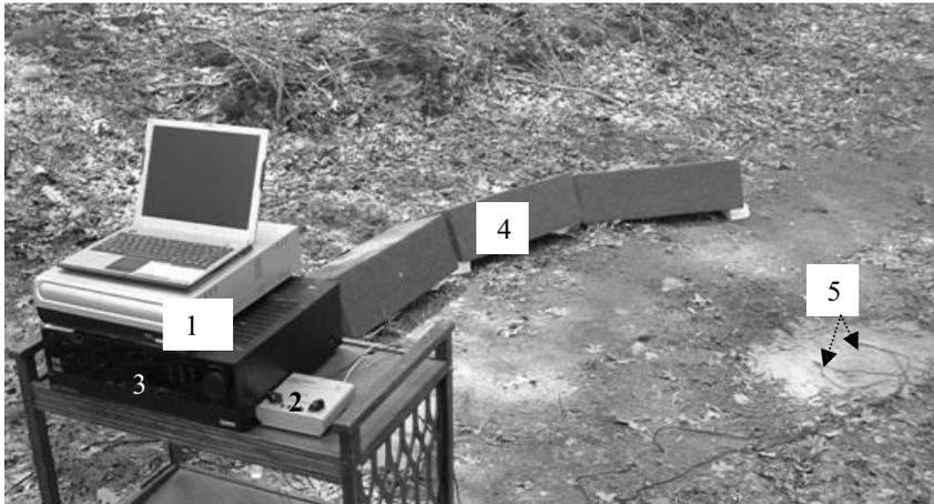
Figure 2. General view of the small scale experimental setup: 1) TRA electronic unit. 2) A microphone preamplifier. 3) Six channel power amplifier. 4) Speakers. 5) Accelerometers.
