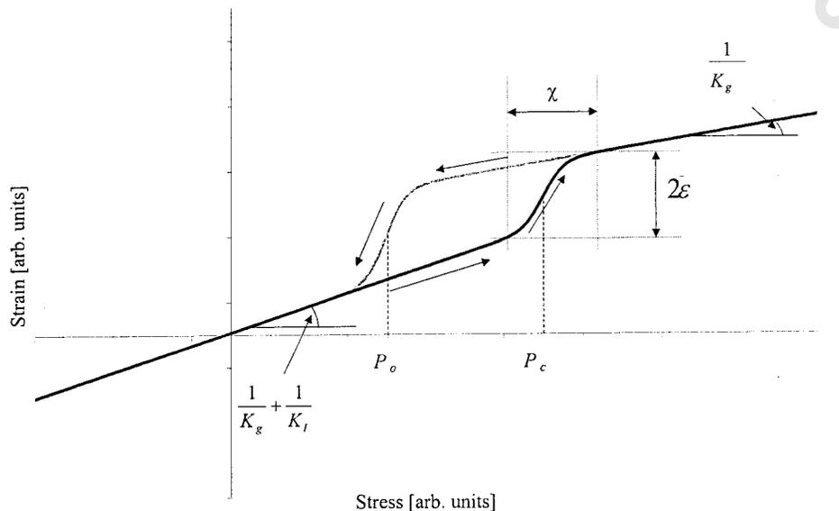
FIG. 3. A continuous micromodel illustrating the stress–strain behavior of a lattice cell characterized by a set of six “elastic” parameters:  $K_g$ ,  $K_I$ ,  $P_0$ ,  $P_c$ ,  $\kappa$ , and  $\chi$ .
