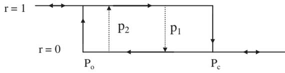
**Figure 2.** Dependence of the state variable  $r$  on the applied pressure  $P$ . The dashed arrows represent the transition rates between the two states  $r = 1$  and 0.
