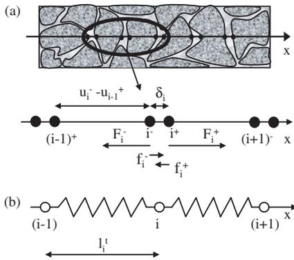
**Figure 1.** (a) One-dimensional lattice representation of the bar. The black dots represent the sub-nodes delimiting the HMU's. (b) Simplified lattice with varying spring rest-lengths  $l_i(t)$ .
