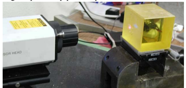
Figure 2. Glass sample with the laser detector.
