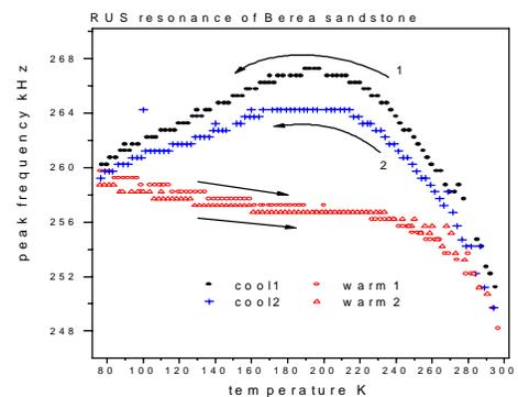
FIGURE 1. The centre frequency dependence of one sandstone resonance over two temperature cycles to 77K
