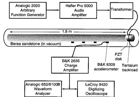
FIG. 1. Experimental setup: Block diagram shows source driver and one detector channel.
