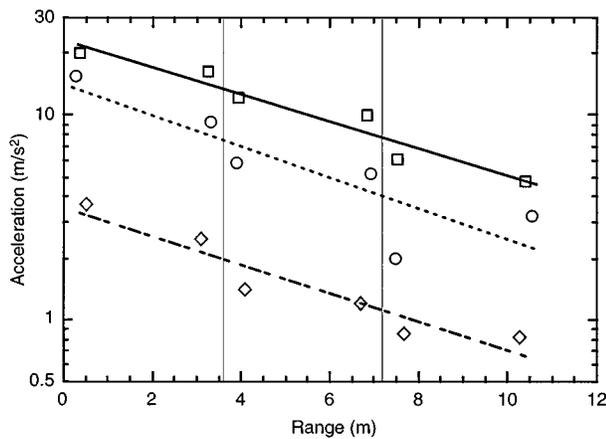
FIG. 4. Peak acceleration values for an initial tone burst and its five later (multiple reflection) arrivals. Squares represent data taken at an accelerometer 28 cm from the source, circles 35 cm from the source, and diamonds 50 cm from the source. Solid, dotted, and dash-dotted lines represent least squares fits to each position, respectively. Vertical lines at 3.6 and 7.2 m represent points where the tone burst is reflected from the source end.
