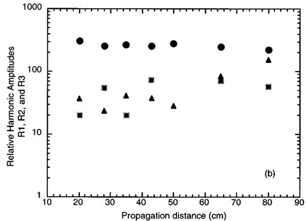
FIG. 9. Spectral ratios as a function of propagation distance for fundamental (circles), second (squares), and third (triangles) harmonics. Source frequencies were (a) 12 kHz and (b) 13 kHz, and source strain amplitude estimated at  $3 \times 10^{-7}$ . All data were taken with the rod in a vacuum of at least 10 mTorr.
