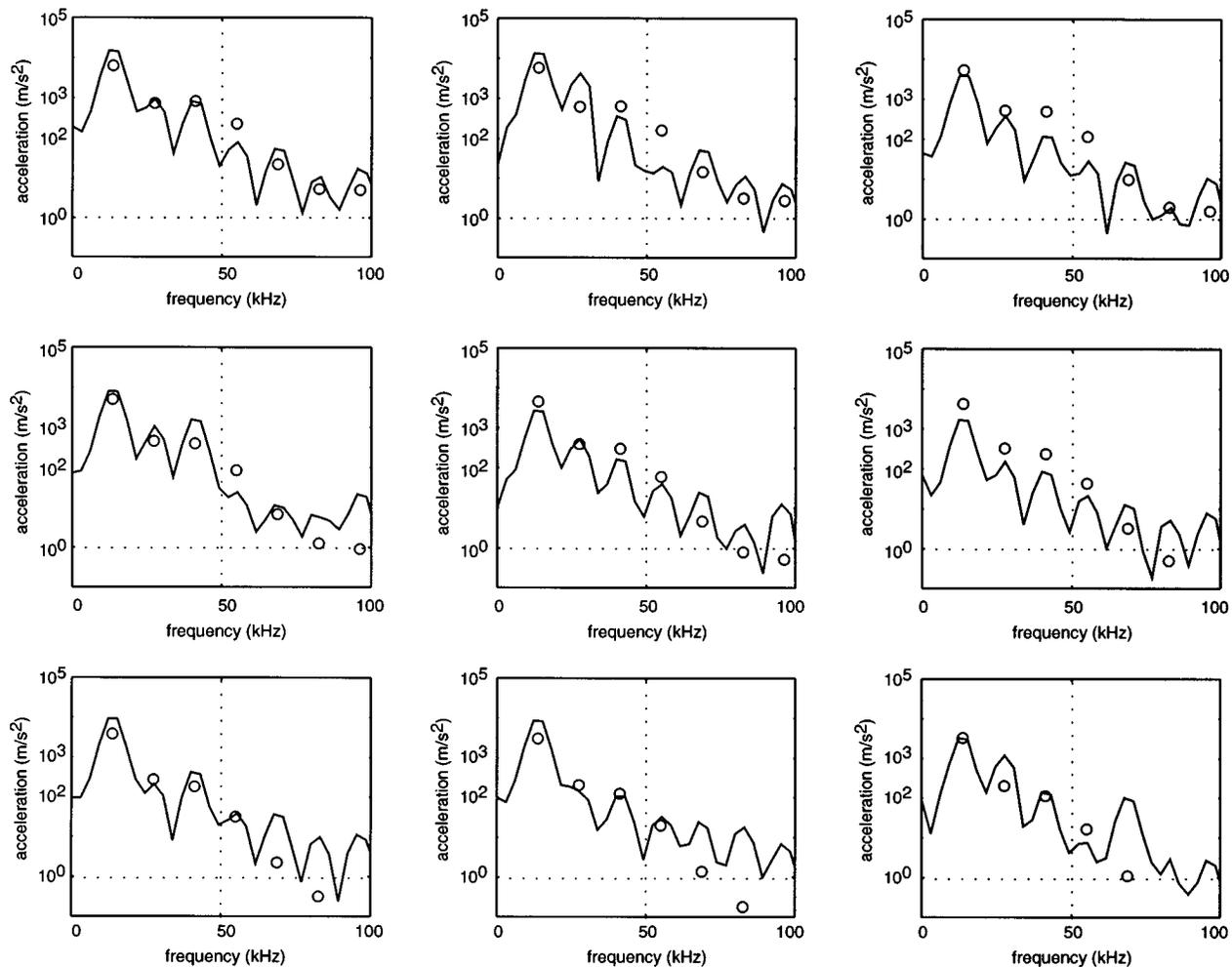
FIG. 7. Model calculations (circles) and measured acceleration spectra (solid lines) for an intense tone burst traveling down the large sandstone rod. Order of spectra is left to right, the upper left hand corner corresponding to the spectrum taken 2.5 cm from the source. Pinducers are separated by 5 cm thereafter.
