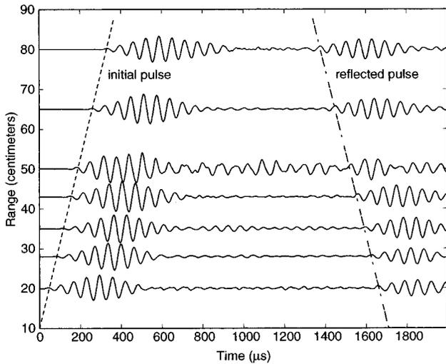
FIG. 3. Typical rangestack used to calculate pulse propagation speed. Data taken from accelerometers on small bar, under vacuum ( $\leq 20$  mTorr) with 0.5-ms tone bursts at 15-kHz source frequency. Each waveform amplitude has been normalized. Dashed line tracks the first arrival of the tone burst and the dot-dashed line tracks its reflection from the far end of the bar.
