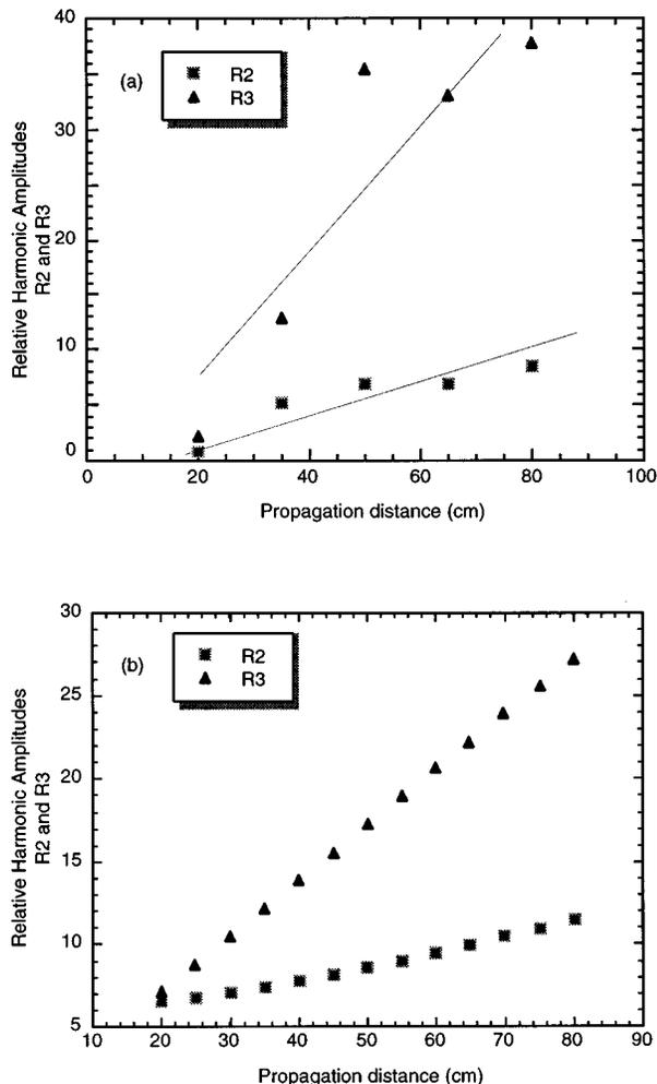
FIG. 10. (a) Spectral ratios as a function of propagation distance for second (squares) and third (triangles) harmonics. Source frequency was 12.4 kHz, source strain amplitude estimated at  $2 \times 10^{-7}$ . Bar was in air. Lines are least-squares fits to guide the eye. (b) Calculated spectral ratios for values of  $\beta$ ,  $\delta$ , and  $Q_E$  of 400,  $2 \times 10^8$ , and 55, respectively.
