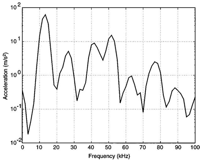
FIG. 8. Source spectrum taken at the source backload of the small bar in air with a B&K 4374 accelerometer. Driving frequency was 12.4 kHz.
