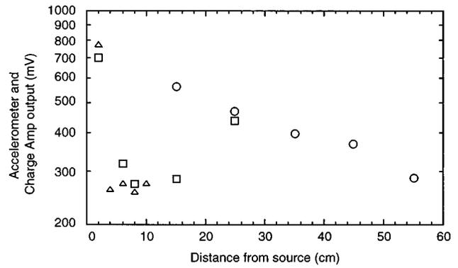
FIG. 5. Output of several accelerometers (oriented to be sensitive to radial  $r$  motion) mounted near the source operating at 12 kHz on the small bar. Different symbols indicate different runs.
