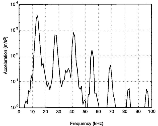
FIG. 6. Spectrum (magnitude) of a large amplitude source signal taken from a B&K 8309 accelerometer mounted on the rear face of the Ta backload. Driving frequency was 13.75 kHz.
