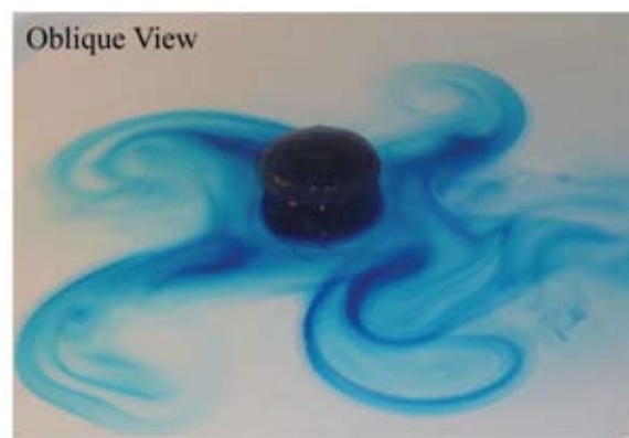
Figure 5. Photographic images of visualization of the flow in (a) the nonrotating experiment and (b) the rotating experiment when the rotation is at 16 revolutions per minute. The blue dye helps visualize the flow of the cold water. In the nonrotating case, the cold water flows outwards but otherwise exhibits little structure. In the presence of rotation, the process of baroclinic instability gives rise to the distinctive multiple spiral-arm structure.
