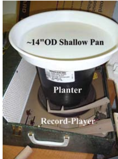
Figure 4. Photograph of the experimental setup. A vinyl record player is used as the rotating table. The planter, with a hole cut in its bottom, accommodates the spindle of the record player and is centered by hand along the axis of rotation. The shallow pan is then hand centered on the planter. Water is used in the shallow pan as the working fluid.
