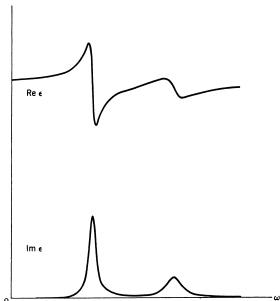
The dielectric constant as a function of frequency.
