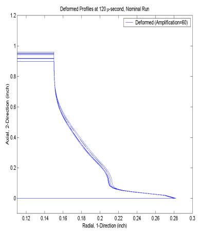
High-strength steel HSLA 100 246 m/s impact velocity
