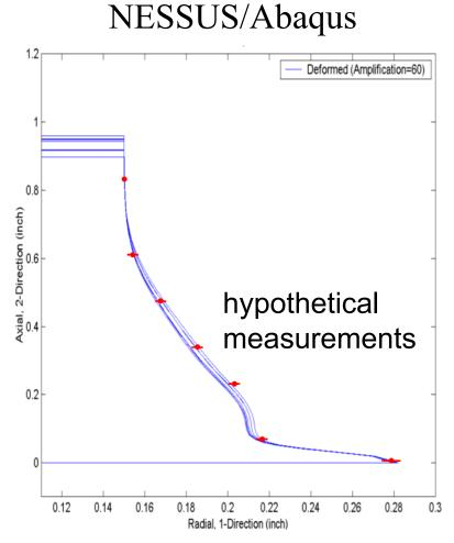
High-strength steel HSLA 100 246 m/s impact velocity
