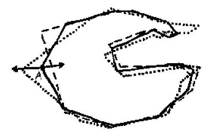
**Figure 1.** An example of how a polygon (solid line) can be distorted by either pushing node A inward (dashed line) or outward (dotted line), assuming that the measurements consist of two orthogonal projections. Note the effect on the overall shape of the object, which indicates the correlations between the polygon vertices.
