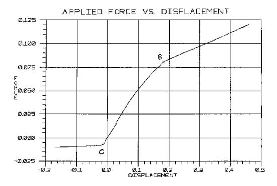
**Figure 2.** Plot of the force applied to node A of the polygon in Fig. 1 versus the resulting displacement of that node. The nonlinear nature of the force-displacement law for this problem is dramatically demonstrated. The configurations shown in Fig. 1 are at the two breakpoints in the curve: the dashed line corresponds to a force of -0.006 (inward) at point C and the dotted line to a force of 0.080 (outward) at B.
