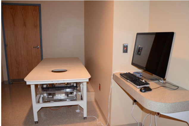
(a) UST scan bed for patient to lie on the bed in the prone position
