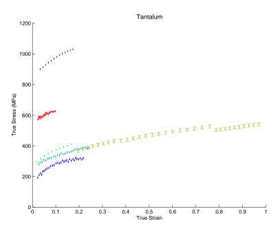
Figure 20: Ta: Sampled data along with  $\pm 1\sigma$  error bars.
