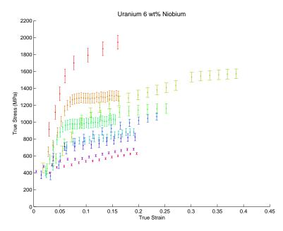
Figure 24: U-6Nb: Sampled data along with  $\pm\,1\,\sigma$  error bars.
