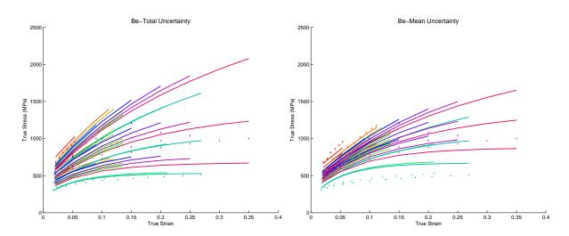
Figure 14: Be: Posterior prediction intervals from the hierarchical model. The left-hand plot is based on  $\eta_{K+1}$  and the right-hand plot is based on  $\eta_0$ . The curves are 0.05, 0.50, and 0.95 point-wise quantiles from the MCMC output.
