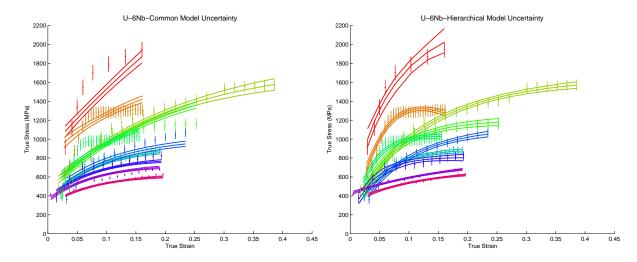
Figure 25: U-6Nb: Point-wise posterior prediction intervals from the common model fit, left-hand plot, and the hierarchical model fit, right-hand plot. The curves are 0.05, 0.50, and 0.95 point-wise quantiles from the MCMC output. The curves in the right-hand plot are based on the  $\eta_i$ s.
