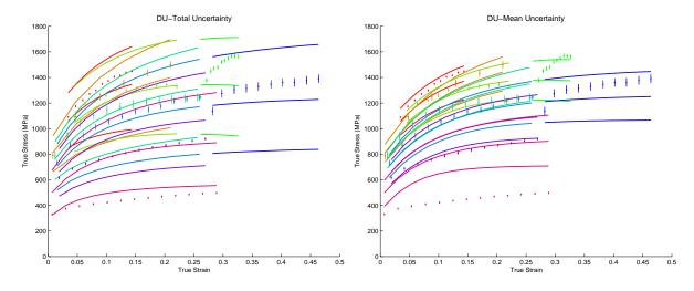
Figure 19: DU: Posterior prediction intervals from the hierarchical model. The left-hand plot is based on  $\eta_{K+1}$  and the right-hand plot is based on  $\eta_0$ . The curves are 0.05, 0.50, and 0.95 point-wise quantiles from the MCMC output.
