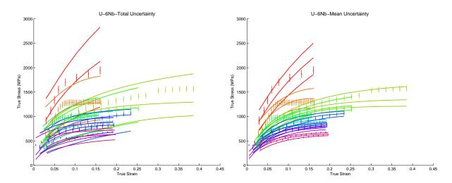
Figure 27: U-6Nb: Posterior prediction intervals from the hierarchical model. The left-hand plot is based on  $\eta_{K+1}$  and the right-hand plot is based on  $\eta_0$ . The curves are 0.05, 0.50, and 0.95 point-wise quantiles from the MCMC output.
