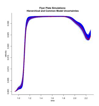
Figure 5: Flyer plate traces corresponding to the final distribution of PTW parameters from the hierarchical model (blue) and common model (red). Each set contains 500 velocity curves. There is very little variability in the common model traces relative to the hierarchical model traces.
