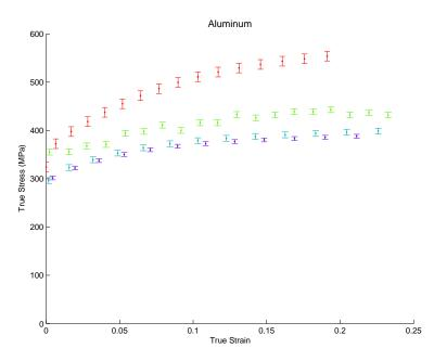
Figure 7: Al: Sampled data with  $\pm 1 \sigma$  error bars.
