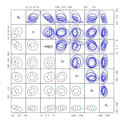
Figure 26: U-6Nb: Approximate 95% posterior probability regions. The blue ellipses in the upper right correspond to the  $\eta_i$ s, one for each data set. The broken black ellipses and the solid black ellipses correspond to  $\eta_0$  and  $\eta_{K+1}$ , respectively, from the hierarchical model fit. The cyan ellipses in the lower left correspond to  $\eta_0$  from the common model fit.
