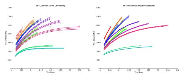
Figure 12: Be: Point-wise posterior prediction intervals from the common model fit, left-hand plot, and the hierarchical model fit, right-hand plot. The curves are 0.05, 0.50, and 0.95 point-wise quantiles from the MCMC output. The curves in the right-hand plot are based on the  $\eta_i$ s.
