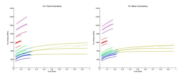
Figure 23: Ta: Posterior prediction intervals from the hierarchical model. The left-hand plot is based on  $\eta_{K+1}$  and the right-hand plot is based on  $\eta_0$ . The curves are 0.05, 0.50, and 0.95 point-wise quantiles from the MCMC output.
