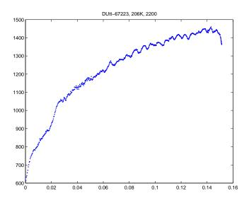
Figure 15: Plot of data obtained from Hopkinson-bar experiment with depleted uranium at 206K and a strain rate of 2200/s.
