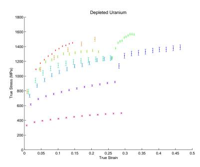
Figure 16: DU: Sampled data with  $\pm 1\sigma$  error bars.
