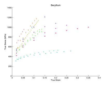
Figure 11: Be: Sampled data with  $\pm 1 \sigma$  error bars.
