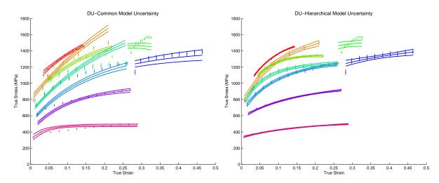
Figure 1: Fitted values and uncertainties for each of the 9 DU Hopkinson-bar experiments. The left-hand plot shows the posterior mean and point-wise 90% uncertainty bounds under the common model. The right-hand plot shows the posterior mean and point-wise 90% uncertainty bounds under the hierarchical model.
