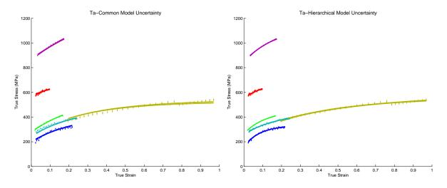
Figure 21: Ta: Point-wise posterior prediction intervals from the common model fit, left-hand plot, and the hierarchical model fit, right-hand plot. The curves are 0.05, 0.50, and 0.95 point-wise quantiles from the MCMC output. The curves in the right-hand plot are based on the  $\eta_i$ s.
