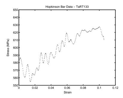
Figure 6: Plot of data obtained from Hopkinson-bar experiment done on tantalum at room temperature and a strain rate of 1300  $s^{-1}$ .
