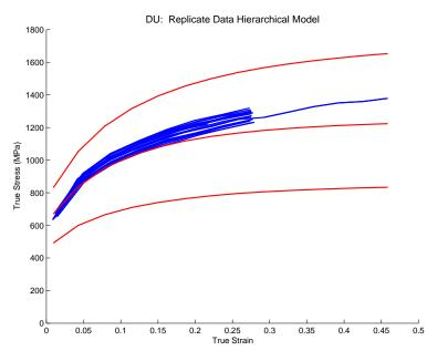
Figure 3: Estimated prediction uncertainties under the hierarchical modeling framework. The hierarchical model uses individual parameter uncertainties to determine combined uncertainty on the PTW parameters, which results in wider prediction intervals. The top and bottom red curves are point-wise 90% uncertainty bands and the middle red curve is the mean.
