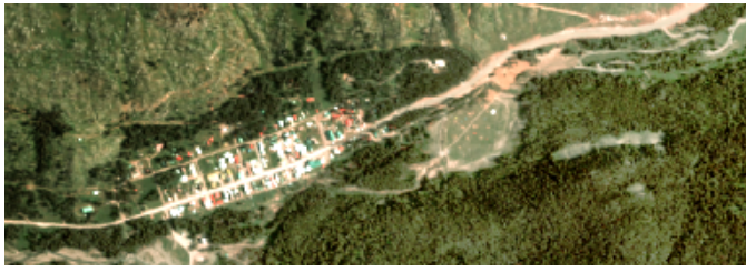
Fig. 3. Bands 3, 5, and 15 of the 128-band hyperspectral image of Cooke City, Montana, are combined into blue, green, and red channels, respectively, of this color image.
