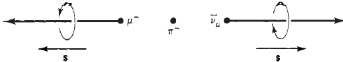
Pion decay at rest with resulting helicity. (Griffiths: Particle Phys)
