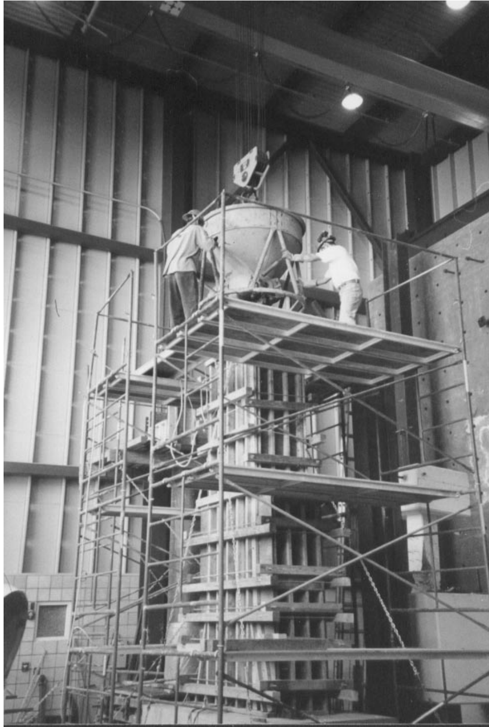
Figure 6.2: The laboratory as a construction site: A technician and a graduate student pour concrete into wooden forms to cast a test specimen. Photograph by the author.
