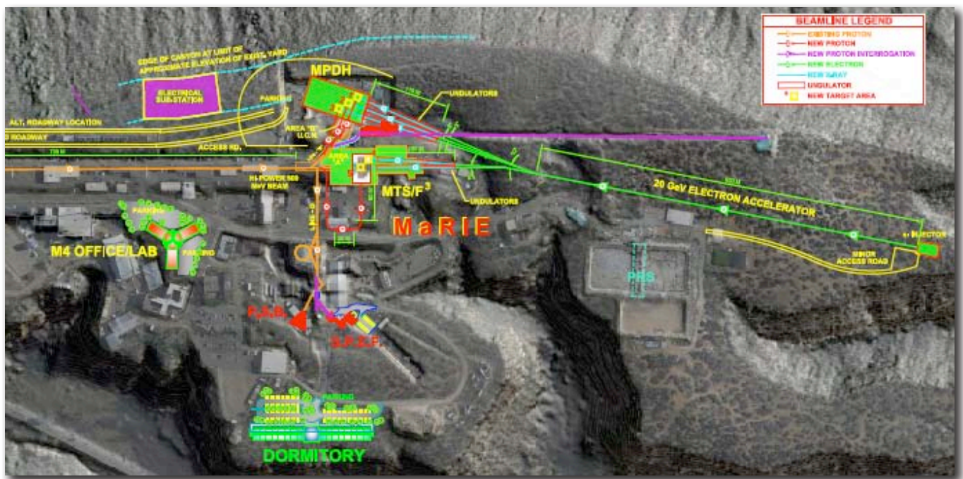
Figure 1. The MaRIE conceptual design incorporates a new XFEL and a LANSCE proton beam power upgrade.
