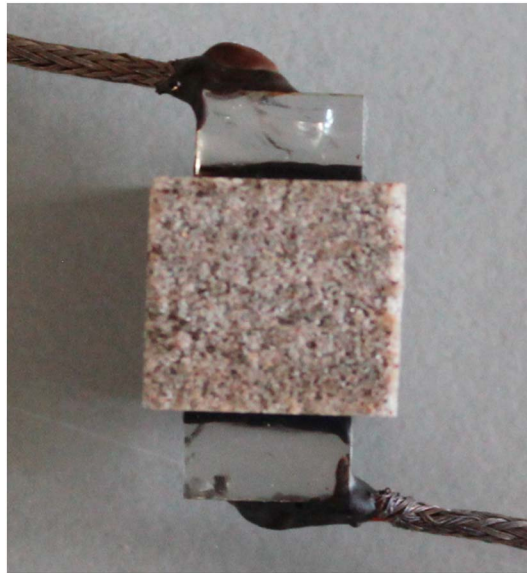
Figure 1. The \text{LiNbO}_3 transducers attached to opposing faces of the 9.13 \times 6.65 \times 8.32 mm Berea sandstone sample using high-temperature epoxy.
